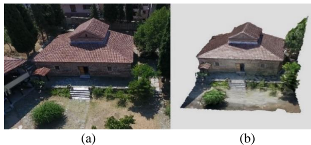
Fig. 2. The church of Saint Nicholas Orphanos. (a) An RGB image captured from a drone. (b) Visualization of the 3D reconstructed model. Copyright Hellenic Ministry of Culture and Sports (L. 3028/2002)
