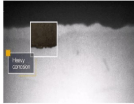
Figure 1. X-ray image that depicts corrosion
