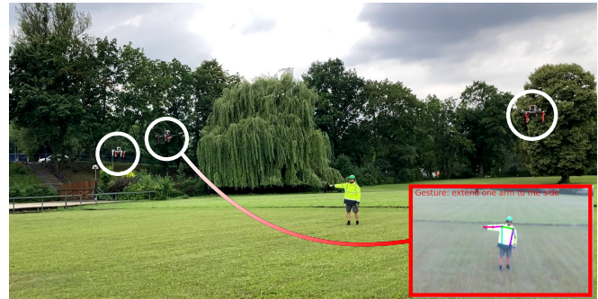
Fig. 1: Snapshot showing the gesture-based interaction between a human worker and a team of three UAVs.
