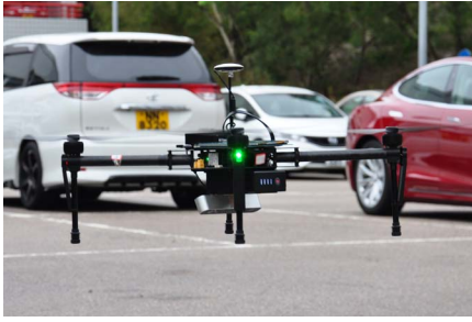
Fig. 5: Experimental set-up for acquiring stereo road images.
