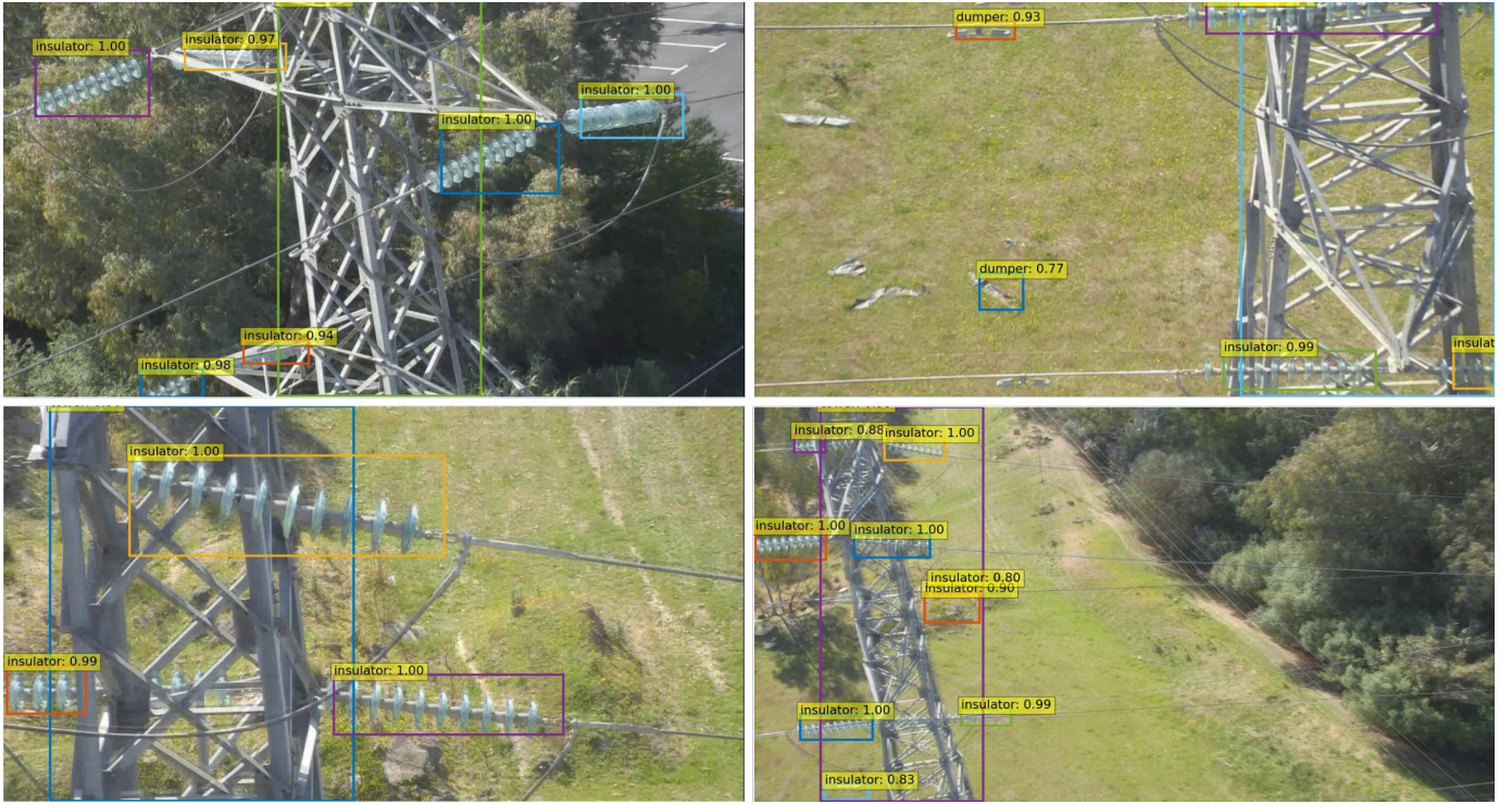
Fig. 2. Image samples of our AERIAL-CORE powerline inspection dataset and elements (e.g. insulators, dumpers and electric towers) detected by DETR detector. The dataset contains a high variety of image shots. Images on the right part of the figure demonstrate the challenges of powerline inspection as some of the objects, e.g. dumpers, are falsely detected or are too small ( 32^2 < \text{area} < 96^2 pixels) against an indistinguishable background.
