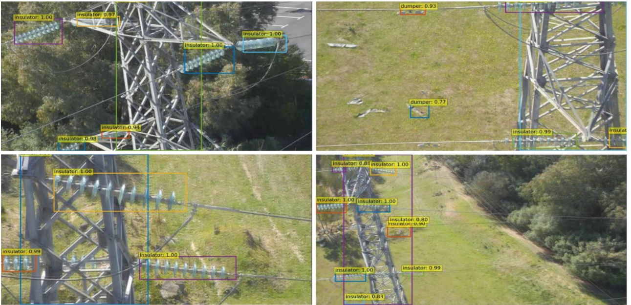
Figure 1. Image samples of the AERIA-CORE powerline inspection dataset and elements detected by DETR detector. The dataset contains a high variety of image shots.
