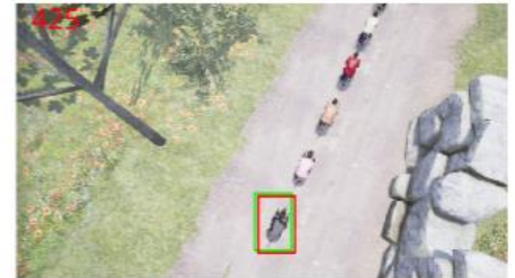
(c) Video frame from UAV 2, following the desired target with a VTS CMT.
