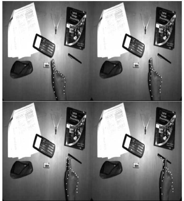
Figure 2: Hand tracking sequence – Kullback-Leibler distance based tracking refinement scheme.
