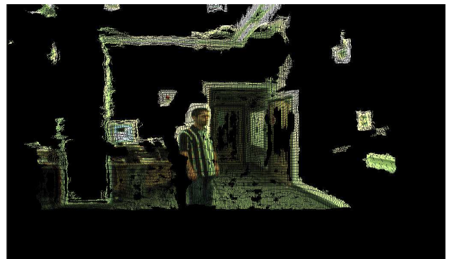
Fig. 4. 3D reconstruction of a single frame captured by the reference camera
