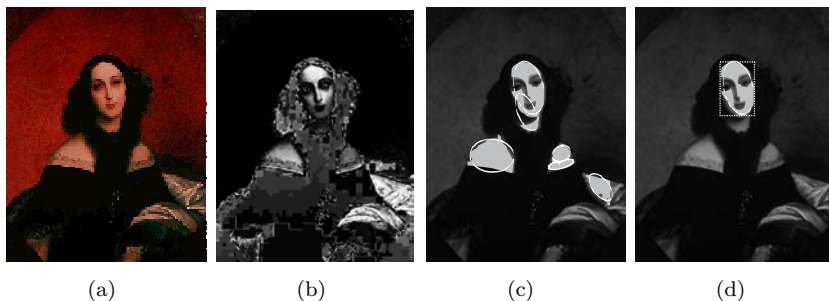
Figure 1. Illustration of individual steps of the method. a) Original image. b) After color pixel segmentation. c) Ellipses fitted to the segmented candidate regions. d) Final output.
