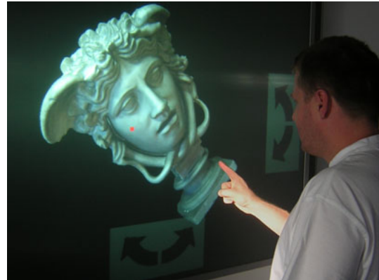
Figure 3: Interaction with a three-dimensional object using virtual buttons to point at for rotation (3D-Model by courtesy of the Picture Gallery of the Academy of Fine Arts Vienna).
