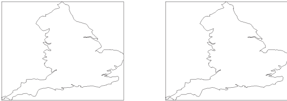
Fig. 2. Original (left) and watermarked (right) polygonal line (outline of England obtained from GIS data).
