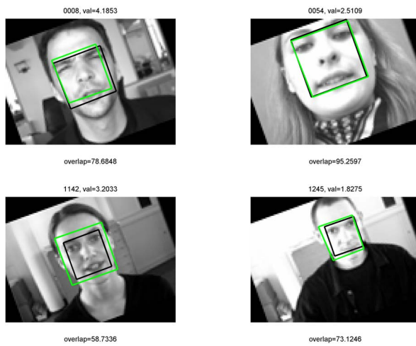
Fig. 3. Output of our face detector on a number of 20^\circ rotated images from the BioID Database.
