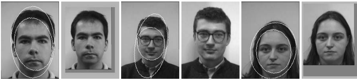
Figure 2. Facial images collected under variable recording conditions. The first, third and fifth images are original ones. The second, fourth and sixth images are normalized ones. The best ellipses determined by the algorithm are drawn on the original images.
