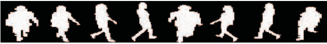
Fig. 5. An eight-view posture frame of action walk. The first posture frame corresponds to the frontal view and the order is clock-wise.
