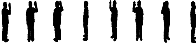
Fig. 3. Projected silhouettes of the 3D mesh models onto the respective image planes for 8 camera views.
