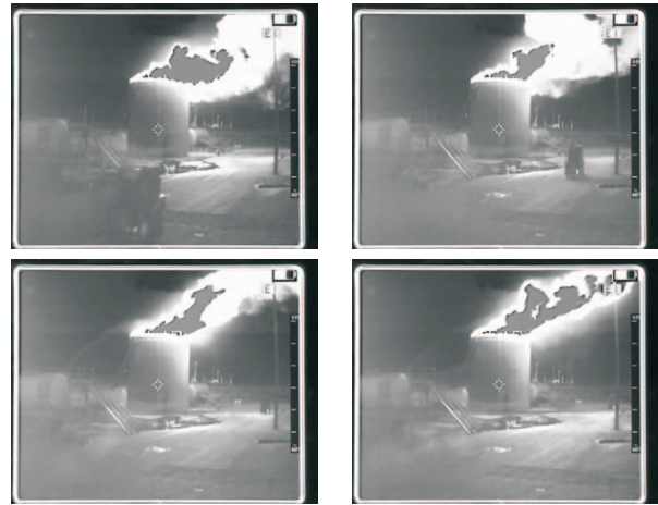
Fig. 9. Consecutive frames from a thermal video to detect fire presence.
