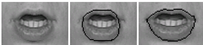
Fig. 6. Outer lip contour extraction example for M2VTS database. From left to right: the original mouth image; outer lip contour tracked with our algorithm; outer lip contour tracked with B-splines.
