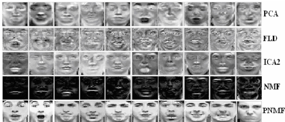
Figure 2. Holistic subspace image representation. From top to bottom, each row depicts 10 basis images ( \mathbf{Z} ) corresponding to PCA, FLD, ICA2, NMF, and PNMF (degree 7). For PCA the basis images are ordered by decreasing variance, for ICA2 and NMF by decreasing kurtosis. Cohn-Kanade AU-coded facial expression database has been used as image samples.
