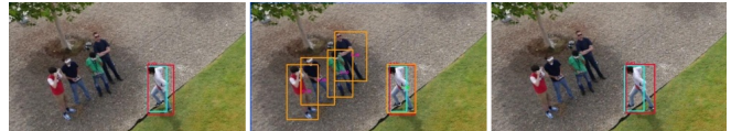
Fig. 1. Example of the proposed joint tracking and tracking framework. During tracker’s \mathcal{T} normal function, the reported bounding box (red) is evaluated by the classifier \mathcal{C} , and a decision is made on whether the reported bounding box corresponds to the correct target (cyan). Based on the classifier’s output, the detector \mathcal{D} predicts possible locations of the target (yellow). The classifier chooses the correct target and tracking continues.
