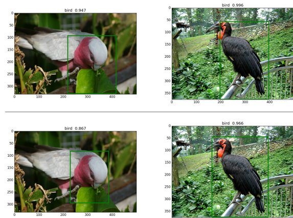
Figure 6: Indicative examples of a class where our model’s precision is worse than the baseline. Upper row: Our model’s detections for the class Bird . Lower row: Baseline’s detections for the class Bird . Our model has improved confidence but the bounding boxes are less accurate.
