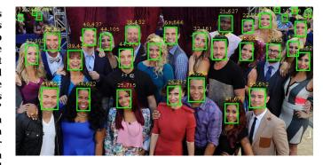
Fig. 1. An example of face detection in various poses and occlusions. The bounding boxes show output of the trained CNN. The scores shown are the result of the last convolutional layer of the face detection stream.
