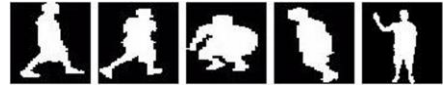
Fig. 2. Posture images depicting five activities observed from various viewing angles. From left to right: walk, run, jump in place, jump forward, and wave one hand.
