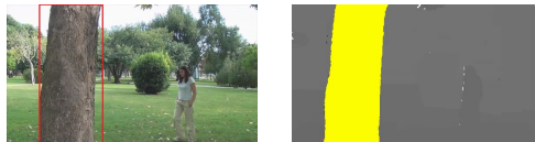
Fig. 3. A bent window effect example. The ROI that encloses the detected object is marked red. Yellow marked regions have disparity values lower than -15 pixels.
