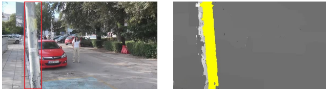
Fig. 2. A bent window effect example. The ROI that encloses the detected object is marked red. The yellow region has disparity values lower than the corresponding threshold.
